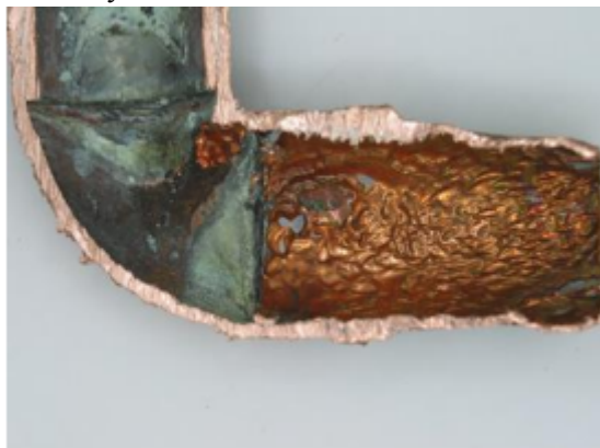
Figure 3. Erosion corrosion Source: Budi Utomo, 2009
