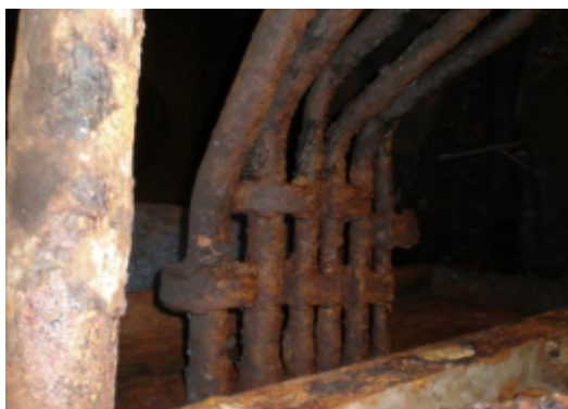
Figure 1. Uniform Corrosion on ballast pipes
